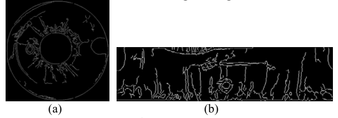
Figure 5. (a) Result of Canny edge detection to Fig.4 (a); (b) Result of Canny edge detection to Fig.4 (b).
